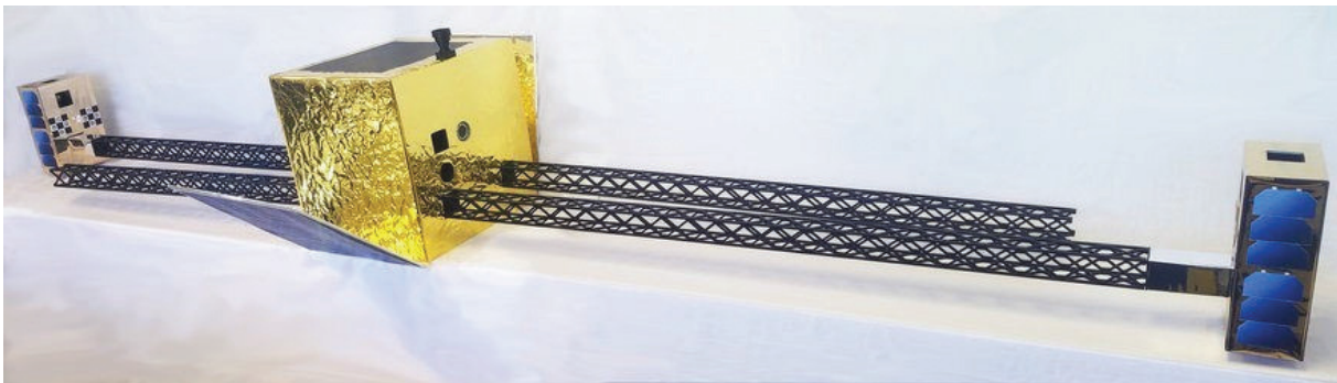
Optimast-SCI, a space assembled interferometer. Using on-orbit assembly and manufacturing, the system will deploy booms up to 50 m long that will allow high angular resolution observations to be made. Credit: Redwire.
